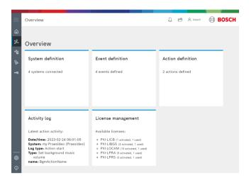
The Intelligent control is a PXI-CORE Edge controller application that offers smart IP-based integration between various Bosch Security and Safety products by making use of the available IP interfaces. It offers flexibility to start activities in a system based on inputs from other connected systems.
