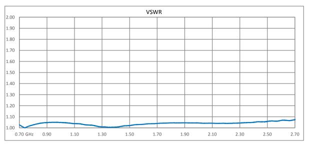
Click the following link (or enter part number in "SEARCH" on website) to obtain additional part information including price, inventory and certifications: Type N F/M Bulkhead Coaxial RF Surge Protector, 698MHz - 2.7GHz, DC Block, 500W, IP67, .005uJ, 40kA, Filter, w/ Bracket TSX-NFM-BF
