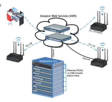
multiple redundant network paths to ensure that console management access is available even if part of the network is down. The dual AC power supply ensures that console management is available even if the primary AC power source fails.
