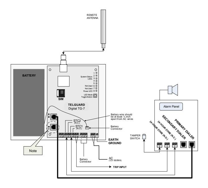
Note: Since there is no Telco connection, there is a single connection for communication—between the Alarm Panel and the TG-7.
