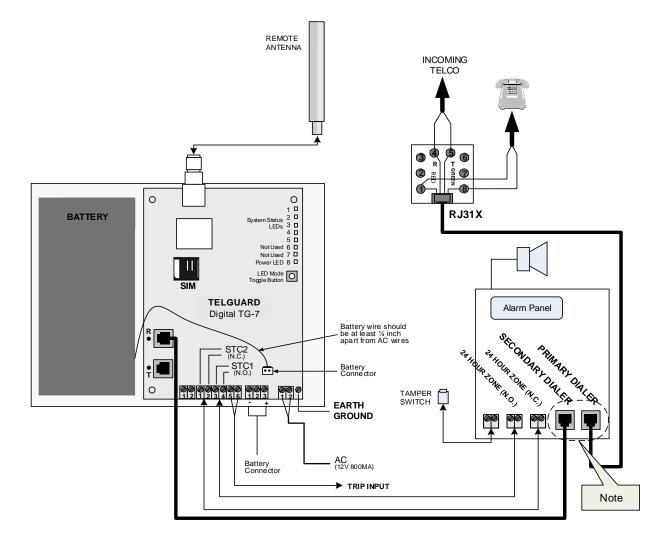
Note: When using this scenario, the use of the primary or secondary dialer to connect to Telco is what determines whether the TG-7 is meant to work as a back-up or primary communicator.
