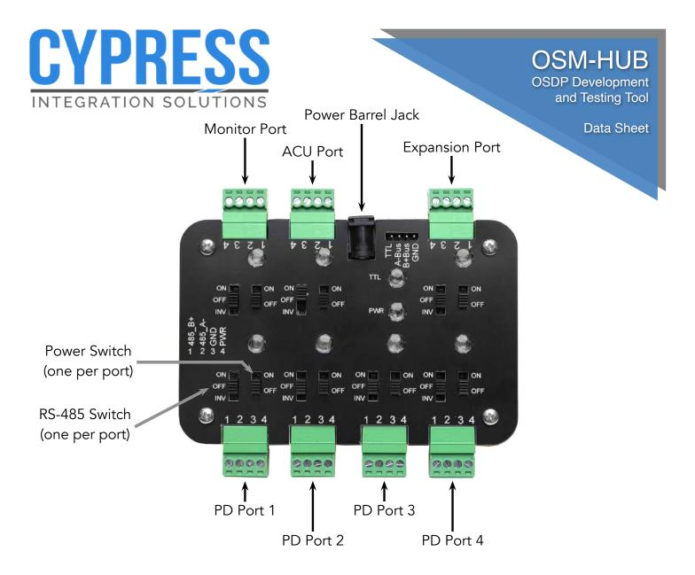
The OSM-HUB is an OSDP developmental and bench-testing tool which passively connects OSDP devices.
