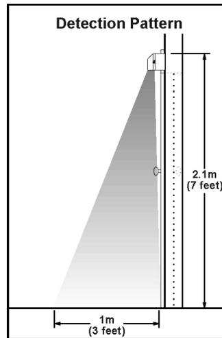
Once the T.REX is installed and the cover replaced, the span and target direction of the detection pattern is set by gently turning the louver direction screws, located just below the detector lens on the barrel. As the adjustment range is about 45°, you must be careful not to turn the louvers too far; stop turning when resistance is felt. The slots on the louver adjusting screws indicate the position of the louver and serve as an adjustment guide. To adjust
