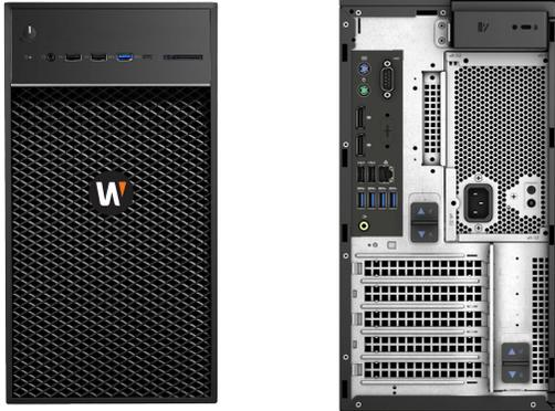
The WRT-P-3101W series dual purpose Wisenet WAVE server and client is built into a compact mini-tower form running Windows 10 IoT Enterprise LTSC or Ubuntu Linux 18.04 LTS. This ready to deploy solution can manage up to 170 Mbps of recording throughput and up to 16TB of storage for a single site or as an addition to your existing Wisenet WAVE system.
