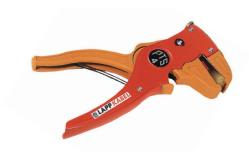
The PTS4 is designed for stripping single conductors from 0.25 mm² (24 AWG) to 4 mm² (12 AWG). It can be used to strip several conductors of the same gauge size simultaneously. The blades are self-adjusting to prevent damage to the conductors. In addition, the pressure of the cutting jaw may be adjusted. Diagonal cutters are also integrated so that cutting and stripping can be done with the same tool.
