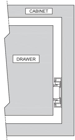
Front view of side mounted slide and 10EL Lock. Lock can be positioned on the right hand as well.
