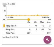
Retries (% of packets) graph: Plots percentage of transmitted packets that are retry packets
