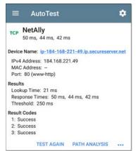
Device Name: DNS name of the device tested
