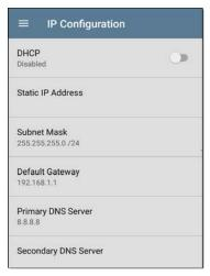
The Static IP address fields for **Subnet Mask**, **Default Gateway**, and **Primary** and **Secondary DNS Servers** only appear if DHCP is disabled. Touch each field to open a pop-up number pad and enter the static addresses as needed. Touch **OK** to save your entries.
