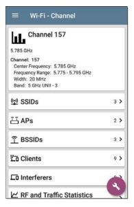
The Channel Details screen displays the channel's Center Frequency under the icon,
