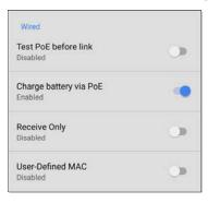
Test PoE before Link: By default, an AutoTest Wired Profile performs the Link test before the PoE test may be able to complete. Enable this setting to make your EtherScope complete the PoE test before the Link test. Enabling this setting forces PoE negotiation to be completed before establishing link, improving compatibility with some switches.
