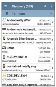
Like in AutoTest and other EtherScope screens, the icons in Discovery change color to indicate a Warning or Failure condition. Discovery also displays device icons in Blue to indicate Problem-related information that does not constitute a warning or failure, and Green to indicate that a previous Problem has been resolved. (See the Problem Settings to adjust enabled Problems and thresholds.)
