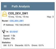
Tapping the <u>blue linked</u> switch name will open a <u>Discovery Details screen</u> for the switch, where the user can investigate the cause of the Warning.
