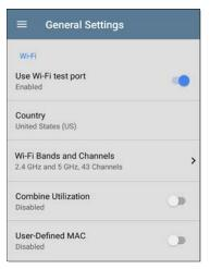
**Use Wi-Fi test port**: Enable or disable Wi-Fi tests, connections, and measurements in the testing apps, including AutoTest Wi-Fi Profiles and the Wi-Fi analysis app.
