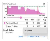
PHY TX Rate (Mbps) graph: Plots the physical transmission rate. The green horizontal dotted line indicates the AP's maximum TX rate.
