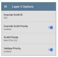
Override VLAN ID: Touch to select or enter a VLAN ID number. The Override VLAN ID function tags frames with a particular VLAN (for example, a VLAN used for voice, video, or data).
