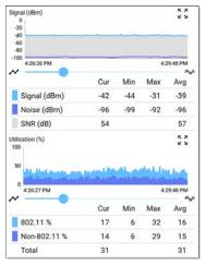
These graphs update in real time and save and display data for up to 24 hours (depending on test type and/or link status).
