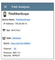
The example image above shows the SSID, Channel, and other Wi-Fi information the EtherScope can display after running a Path Analysis over Wi-Fi.
