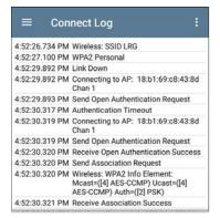
The Connect Log shows the connection log, including driver activity, supplicant, and the DHCP process. The Connect Log can be especially helpful for identifying linking or roaming problems.
