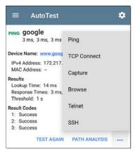
Touch blue links or the blue action overflow icon ••• at the bottom of the test results screens to run the Ping TEST AGAIN, open another testing app, Browse to the Ping target address in your web browser, or start a Telnet or SSH session.
