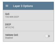
QoS: Select the methodology used on your network: TOS with DSCP (Type of Service with Differentiated Services Code Point or TOS with IP Precedence (legacy). Then, configure the priority using the settings below.
