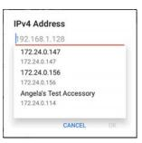
A drop-down list in the IPv4 Address dialog shows all the Test Accessories the EtherScope has discovered through the discovery process, as well as any Test Accessories that are claimed to the same Link-Live organization as your EtherScope.
