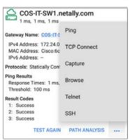
Touch blue links or the blue action overflow icon ••• at the bottom of the test results screens to run the Gateway TEST AGAIN, open another app, Browse to the Gateway's IPv4 Address, or start a Telnet or SSH session to the Gateway.
