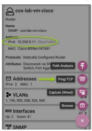
If the Ping/TCP app is opened from this screen, the IPv4 address from the Discovery app is already configured as the Ping/TCP target.
