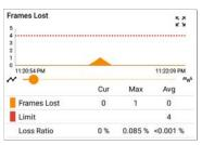
Frames Lost (Up/Down): Frame loss is quantified by the number of frames received subtracted from the number of frames sent.
