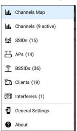
The Wi-Fi app's navigation drawer displays a real-time count (in parentheses) of each wireless component EtherScope has detected. Tap an option to open the corresponding screen.
