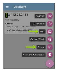
NOTE: You can select **Browse** in the floating action menu to open the Test Accessory's Web Interface, where you can view its status and configure its settings.
