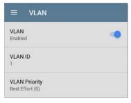
Touch to open the VLAN settings screen. Slide the toggle to the right to enable VLAN testing. Enabling this setting also enables a VLAN test card on the Wired AutoTest results screen. Once enabled, VLAN ID and VLAN Priority fields appear. Touch these fields to open a pop-up number pad and enter the correct ID and priority. Touch OK to save them.
