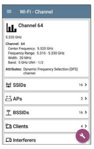
The Channel Details screen above shows how many SSIDs, APs, BSSIDs, Clients, and Interferers are detected on Channel 64. Touch the lower cards in Wi-Fi Details to open a list screen that is filtered for the network component you are examining.
