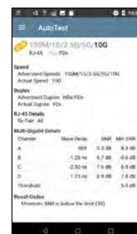
Cabling SNR measurement validates Multi-Gig links
