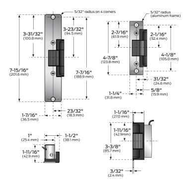
Solenoid power requirements; 12VDC, 0.38 A, 24 VDC, 0.19 A
