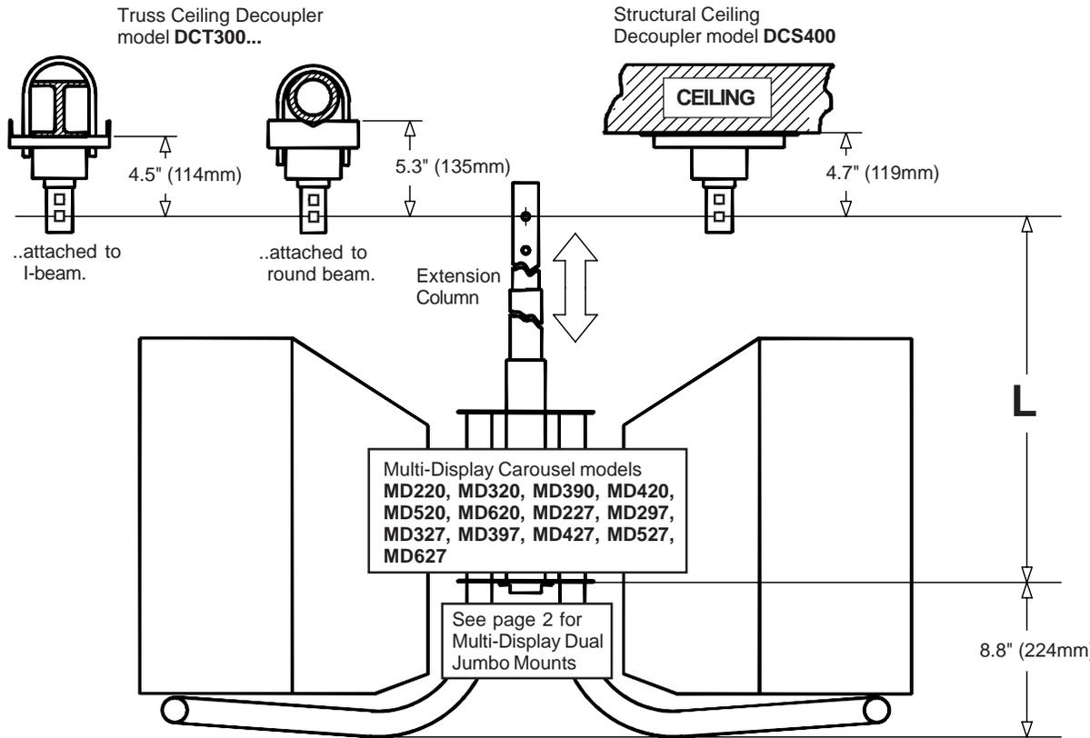
The Extension Column for Multi-Display Mounts is one of three elements required for Multi-Display Ceiling Mount installations. It is available in several lengths which are adjustable at 1" increments (see specifications, above right).
