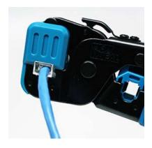
5) Terminate the plug with a modular plug crimper. Use the RJ45 8-position 8-contact cavity.
