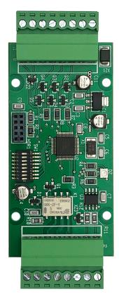
Use the OSM-1000 to simplify OSDP adoption, by upgrading a legacy access control system to the OSDP standard.
