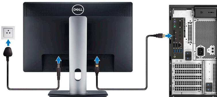
**i** **NOTE:** If you ordered your computer with a discrete graphics card, the HDMI and the display ports on the back panel of your computer are covered. Connect the display to the discrete graphics card.
