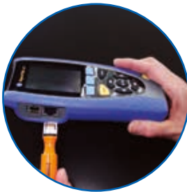
No calibration required plus replaceable RJ45 contacts
