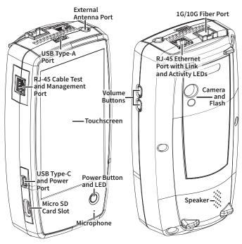
The EtherScope nXG is a rugged, hand-held tool for testing and analyzing copper, fiber, and Wi-Fi networks. It features applications developed by NetAlly for network discovery, measurement, and validation, which are available from the Android Home and Apps screens:
