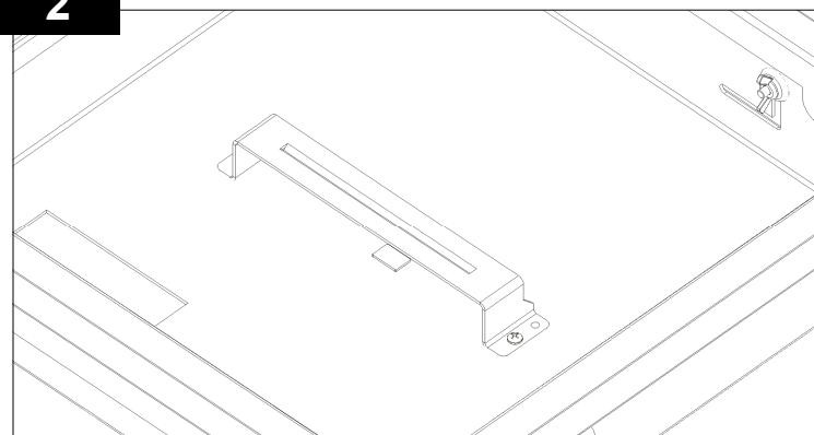
Install the provided T-bar mount into the enclosure.
