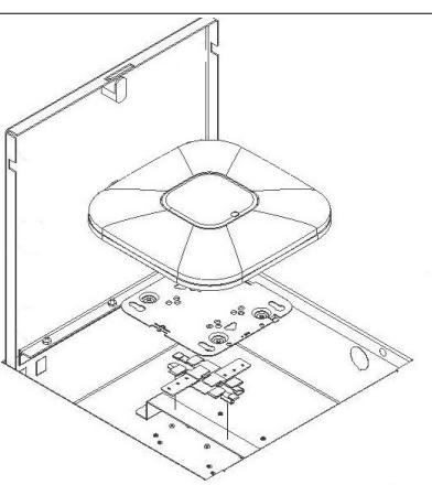
Use the manufacturer's T-bar mount clip to attach the AP to the T-bar mount. Additional components may be required from the AP manufacturer.
