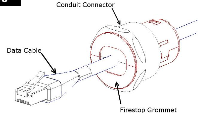
Run the data and power cable (if required) through the conduit connectors located on the sides of the enclosure assembly. Pull the data cable through the conduit connector far enough to allow attachment to the access point. Snap the firestop grommet on to the cable and slide it inside the conduit connector.
