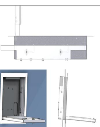
Place the two wall bridges in the mounting position by loosening the four wingnuts inside of the enclosure. The position of the wall bridges will look like the image above. Place the enclosure in the hole cut in the wall or ceiling. Angle the enclosure at 10 degrees with the wall bridges extended towards the bottom. The wall bridges go in first. Once the bottom of the enclosure is in the hole push the enclosure so it is flush with the wall or ceiling.
