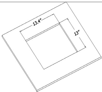
Place the enclosure assembly on the flat work surface with the keyed door unlocked. Remove the necessary knockouts located on the outside edge of the back box to install conduit connectors as required. Install conduit connector. Cut a 13" horizontal x 13.4" vertical opening in the ceiling or wall.
