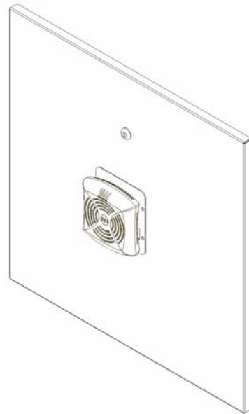
Figure 4 – Proper positioning of AP within the 1068 enclosure. Note that the access point should be located within the AP mount so
