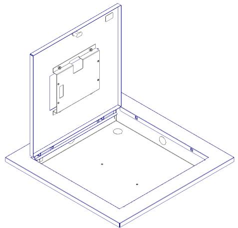
The locking Model 1047-MR series enclosure provides a convenient way to mount and secure Meraki APs in a suspended ceiling or. The AP is mounted in the door. Interchangeable retrofit doors permit vendor and technology migrations, and simplify moves, adds, and changes. UL listed for installation in the plenum space.
