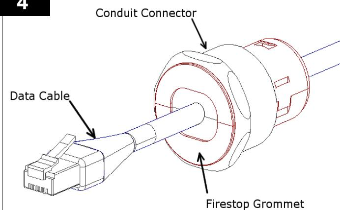
Run the data cable through the conduit connectors located on sides of the *access point enclosure*. Pull the data cable through the conduit connector far enough to allow attachment to the access point (8" - 10"). Snap the grommet on to the cable and slide it inside the conduit connector.
