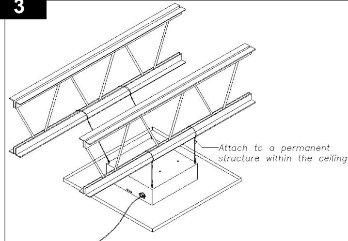
Remove the ceiling tile and replace it with the completed access point enclosure assembly. Use a minimum 12 gauge grid wire to secure the access point enclosure in the ceiling grid. Attach one end of the wire to the eyebolts and the other end to a permanent structure within the ceiling such as a ceiling joist.
