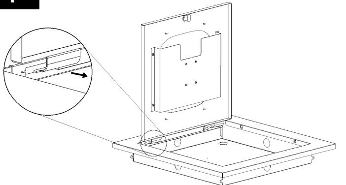
**Find a flat work surface to assemble the ceiling enclosure, access point prior to mounting in ceiling.**
