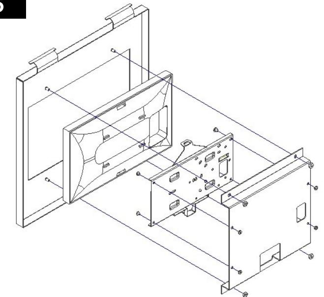
To install the Meraki AP, remove the enclosure's aluminum mounting plate from the door by removing the four (4) nuts that attach the mounting plate.
