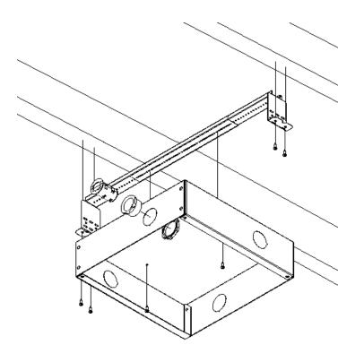
Figure 4 - Installation Into Wall/ Ceiling
