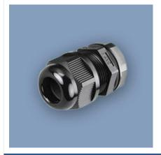
Cord Grip Connector Option - For pre-termination. The polyamide cable gland with split seal A-type clamping design is mounted through a knockout hole or cutout in an enclosure, and provides a watertight seal for preterminated Ethernet cable pass-through. The connector is strain relieving, even after tightening, and supports larger CAT 6a cable diameters.
