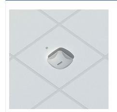
This locking, suspended ceiling tile-like Wi-Tile ™ mount is designed to provide a convenient and aesthetic way to secure Aruba APs in the ceiling. The 1068 features a unique, patented locking mechanism which uses a receiver plate to attach to any of the Aruba enterprise APs. The receiver plate is then locked into the mount. This permits easy migration to new Aruba APs in the future. Textured, white powder-coated steel and aluminum construction.
