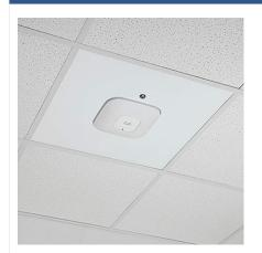
This locking, suspended ceiling tile-like Wi-Tile ™ mount is designed to provide a convenient way to secure Cisco APs in the ceiling. Many of the 106X series AP mounts feature a unique, patented locking mechanism which draws the AP part way into the mount, exposing only the antenna face of the AP, for the ultimate in wireless coverage, aesthetics, and physical security. Textured, white powder-coated steel and aluminum construction.
