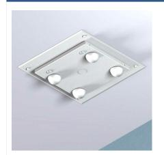
Hard lid ceiling Wi-Tile <sup>™</sup> enclosure protects critical APs, DAS remote units, and public safety equipment with detachable antennas. This water- and dust-proof aluminum enclosure has knockouts in the hinged door for ceiling-mounted antennas or water-resistant bulkhead connectors for antennas. Deep enough for the Cisco 3600 series and other large APs and DAS remote access units with external connectors and up to five antennas. Plenum-rated; provides NEMA 4 dust and water protection.
