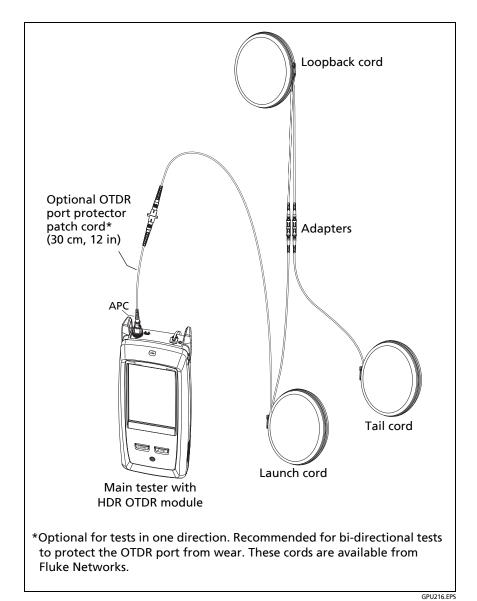
**Figure 183. SmartLoop Launch Compensation Connections**
