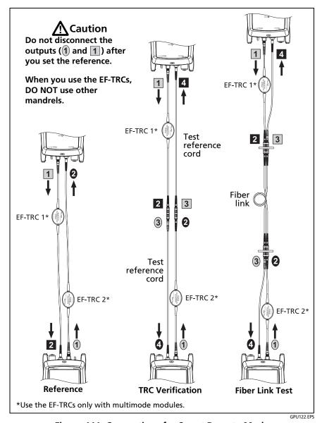
Figure 111. Connections for Smart Remote Mode (1 Jumper Reference, Multimode Fiber)
