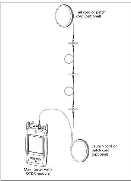
Figure 160. FaultMap Test Connections
