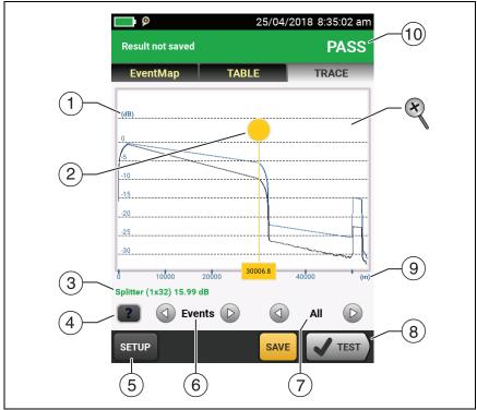
Figure 174. HDR OTDR Trace
