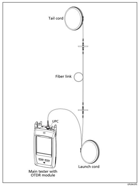
Figure 133. Connections for Launch + Fiber + Tail Compensation
