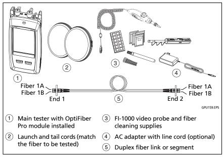
Figure 202. Equipment for the OTDR Project Tutorial
