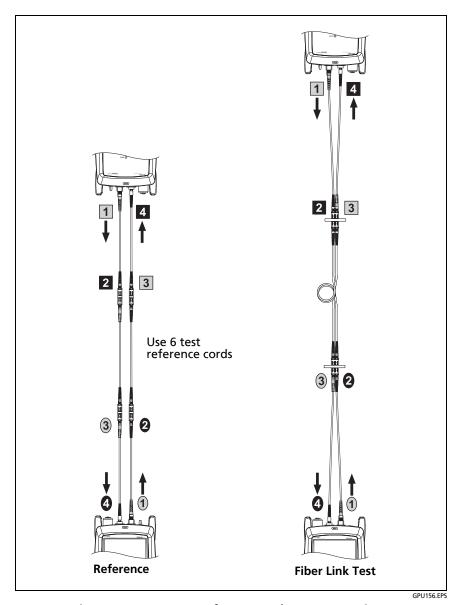
Figure C-3. 3 Jumper Reference and Test Connections (singlemode shown)
