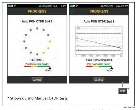
Figure 165. The OTDR Port Connection Quality Gauge and Progress Screen
