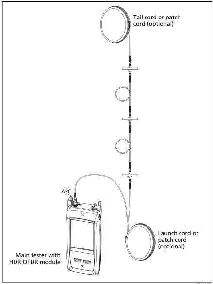
Figure 180. FaultMap Test Connections
