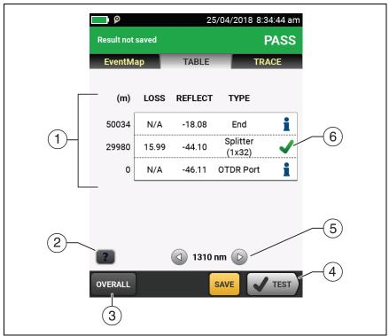
Figure 171. Event Table from an HDR OTDR Test
