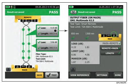
Figure 14. Examples of Fiber Autotest Results Screens
