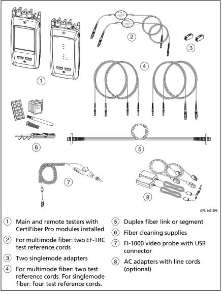
Figure 12. Equipment for the Fiber Certification Tutorial
