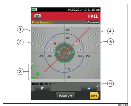
Figure 101. FiberInspector Image with Defect Analysis
