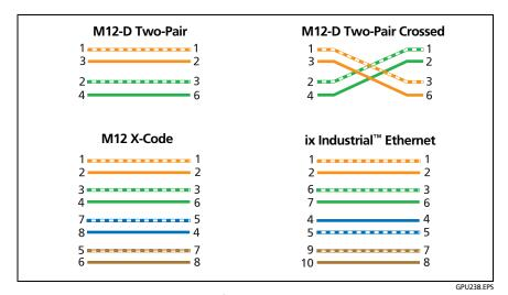
Figure 29. Outlet Configurations - Industrial Ethernet
