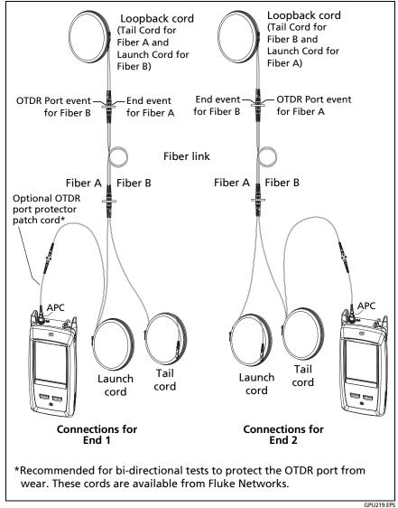
Figure 186. SmartLoop Test Connections for a Bi-Directional Test
