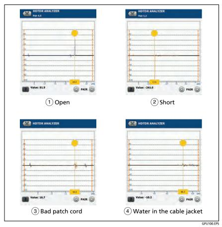
Figure 86. Common Faults Shown on HDTDR Plots
