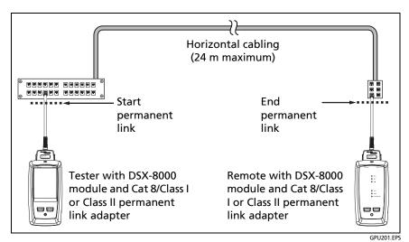
Figure 33. Permanent Link Connections for Cat 8/Class I/II Links
