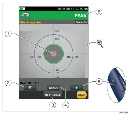
Figure 99. FiberInspector Image with Manual Grading Selected
