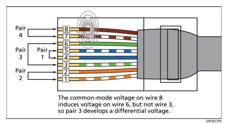
Figure 65. Common-Mode Voltage Converts to Differential-Mode Voltage in an RJ45 Connector
