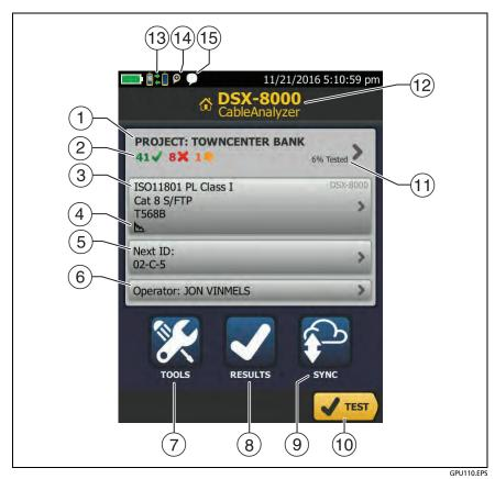
Figure 26. The Home Screen for DSX CableAnalyzer
