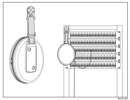
Figure 136. How to Use the Optional TPAK Magnetic Hanger
