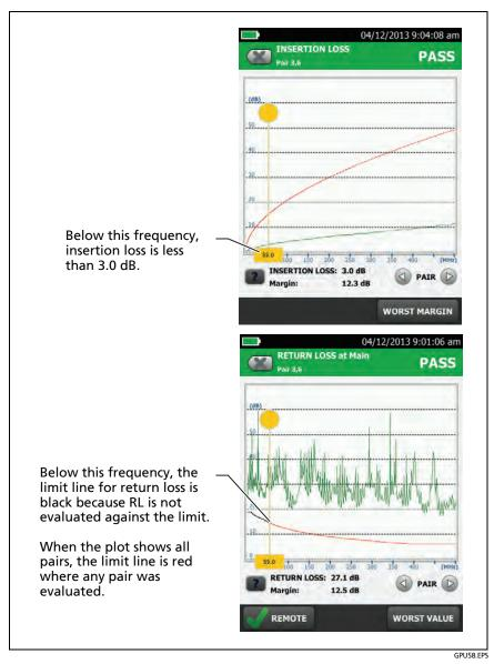
Figure 69. How the 3 dB Rule Shows on Plots
