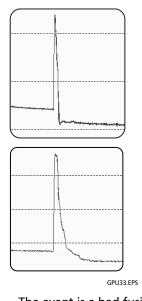
The trace shows a large reflective event with high loss (top) or excessive tailing (bottom). The tester can possibly show it as the End event, though it occurs before the end of the link.
