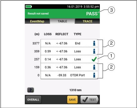
Figure 190. Event Table for a Span
