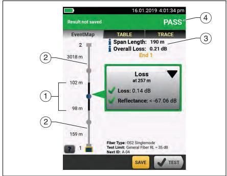
Figure 189. EventMap for a Span
