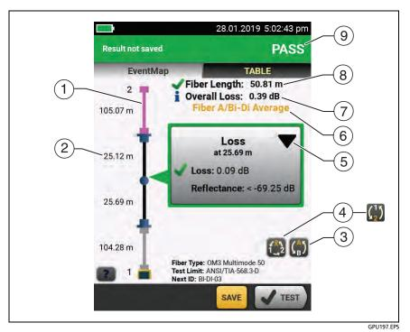
Figure 187. EventMap for Averaged, Bi-Directional SmartLoop Results
