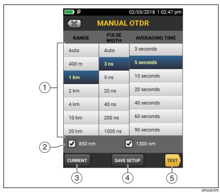
Figure 150. Manual OTDR Screen for Quick Changes to Test Settings
