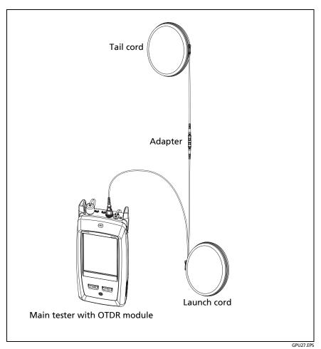
Figure 132. Connections for Launch + Tail Compensation
