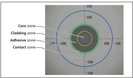
Figure 100. Zones on a Fiber Endface
