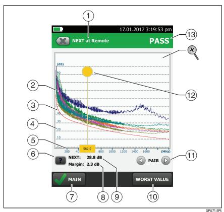
Figure 44. Plot Screen for a Frequency-Domain Test
