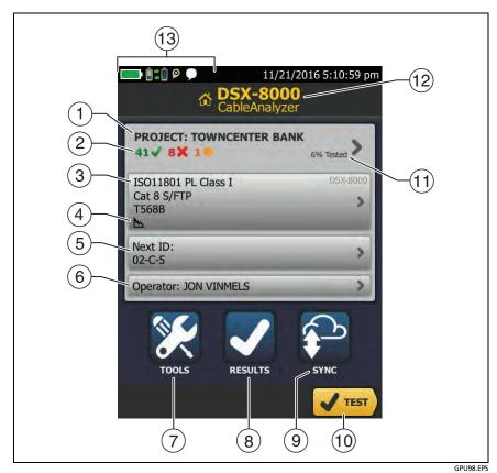
Figure 6. The HOME Screen (DSX CableAnalyzer screen shown)
