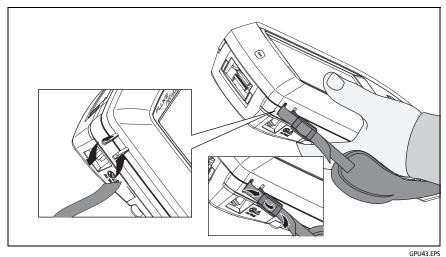
Figure 8. How to Install a Strap and Use the Hand Strap
