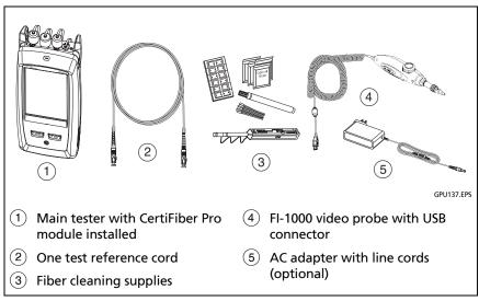
Figure 124. Equipment for Power Meter Measurements
