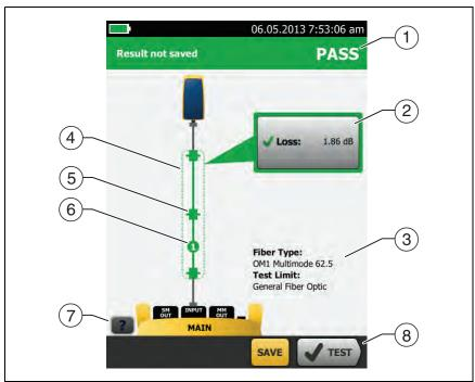
Figure 122. Result for Far End Source Mode
