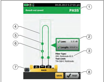
Figure 118. Result for Loopback Mode
