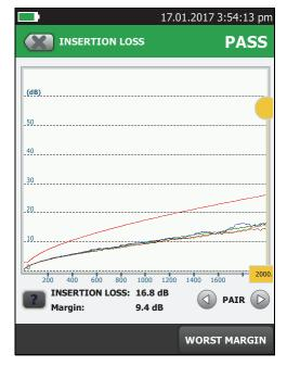
Figure 47. Twisted Pair Insertion Loss Plot
