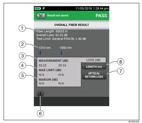
Figure 172. HDR OTDR OVERALL FIBER RESULT Screen
