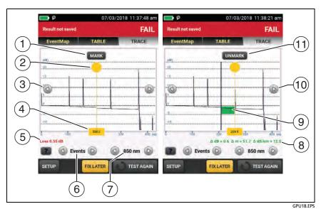
Figure 149. How to Use the Measurement Cursor on the ODTR Trace
