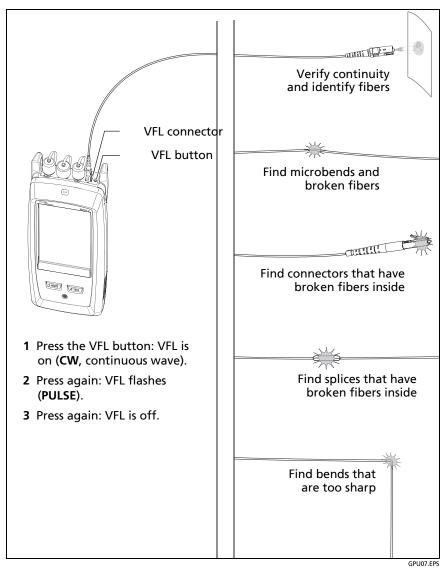
Figure 193. How to Use the Visual Fault Locator
