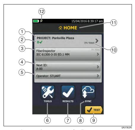
Figure 95. The HOME Screen for FiberInspector Tests
