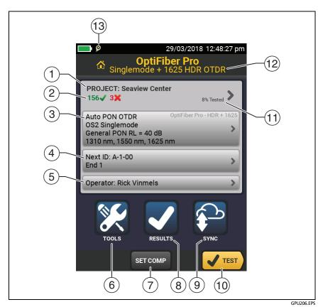
Figure 164. The HOME Screen for OptiFiber Pro HDR Modules
