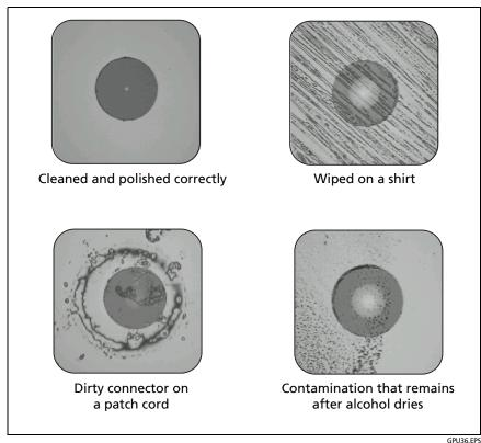
Figure 91. Examples of Clean and Dirty Fiber Endfaces
