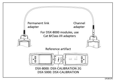
Figure 27. Reference Connections for Twisted Pair Cable
