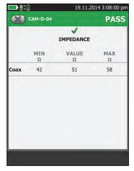
Figure 81. Coaxial Impedance Results
