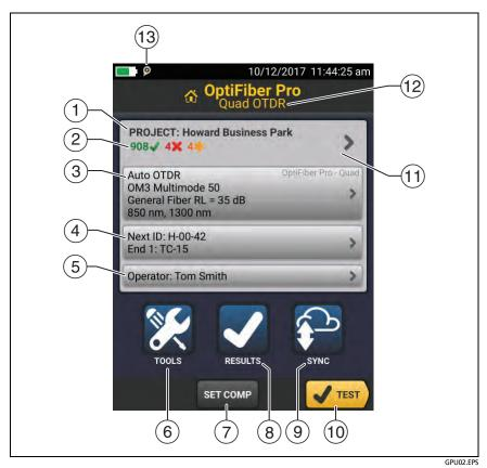
Figure 130. The HOME Screen for OptiFiber Pro Modules
