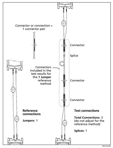
Figure 109. How to Count the Numbers of Connectors, Splices, and Jumpers
