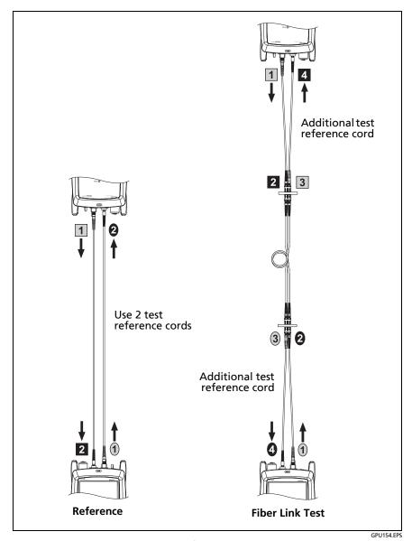
Figure C-1. 1 Jumper Reference and Test Connections (singlemode shown)
