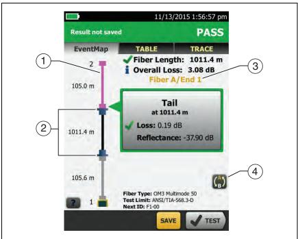
Figure 185. EventMap from a SmartLoop Test
