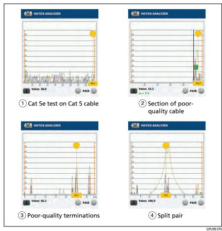
Figure 89. Typical Faults Shown on HDTDX Plots
