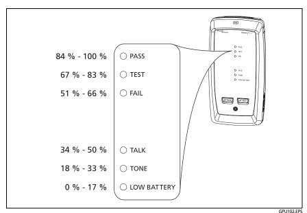
Figure 3. LEDs Show the Remote's Battery Status
