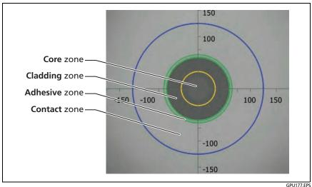
Figure 207. Zones on a Fiber Endface
