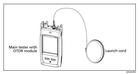
Figure 131. Connections for Launch Only Compensation
