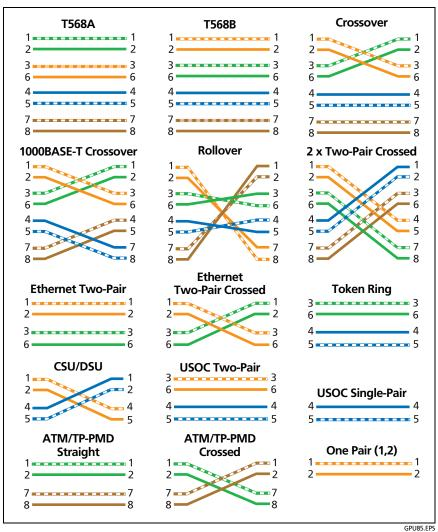
Figure 28. Outlet Configurations - RJ45
