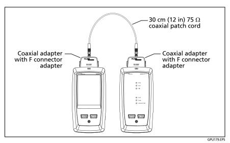
Figure 75. Reference Connections for Tests on Coaxial Cabling
