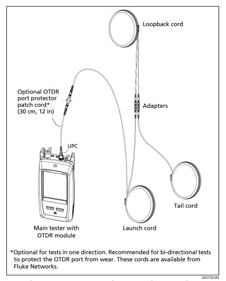
Figure 154. SmartLoop Launch Compensation Connections
