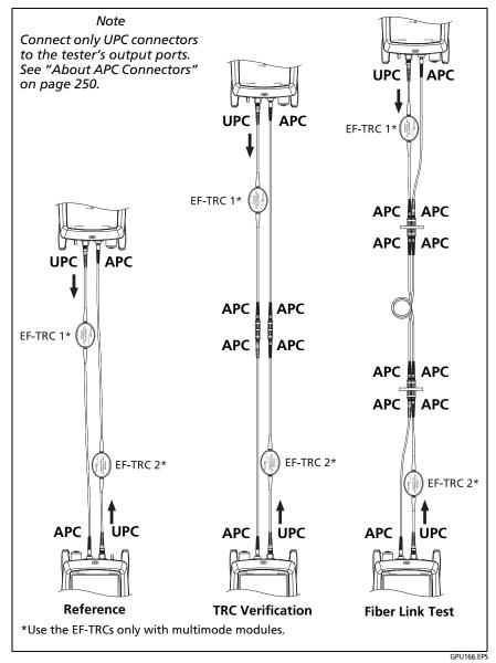
Figure 107. TRCs Necessary for Links with APC Connectors
