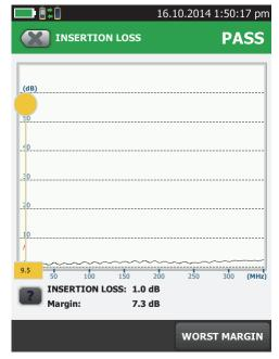
Figure 82. Coaxial Insertion Loss Results
