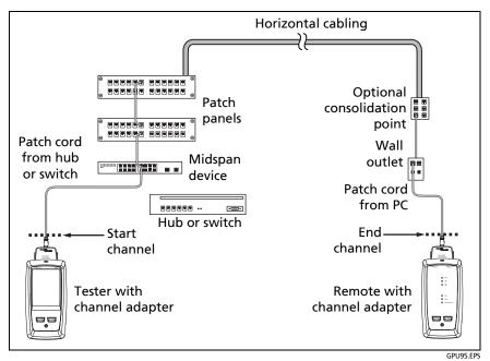
Figure 72. Channel Connections Through a PoE Device
