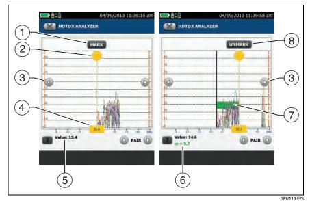
Figure 90. How to Use the Measurement Cursor on the HDTDR or HDTDX Plot
