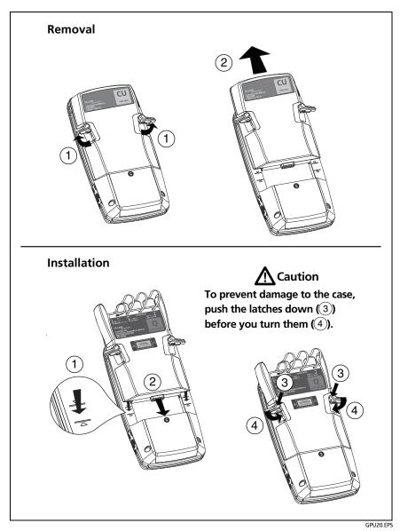
Figure 9. How to Remove and Install a Module
