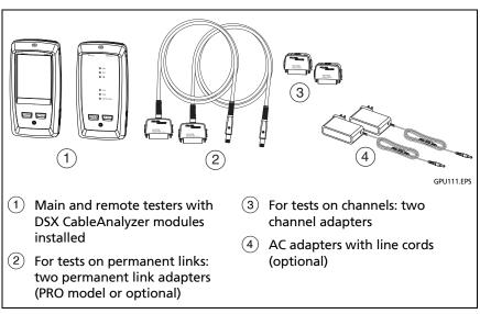
Figure 30. Equipment for Autotests on Twisted Pair Cable
