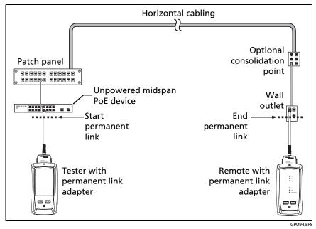
Figure 71. Permanent Link Connections Through a PoE Device
