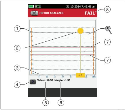
Figure 87. HDTDR Plot for Coaxial Cable
