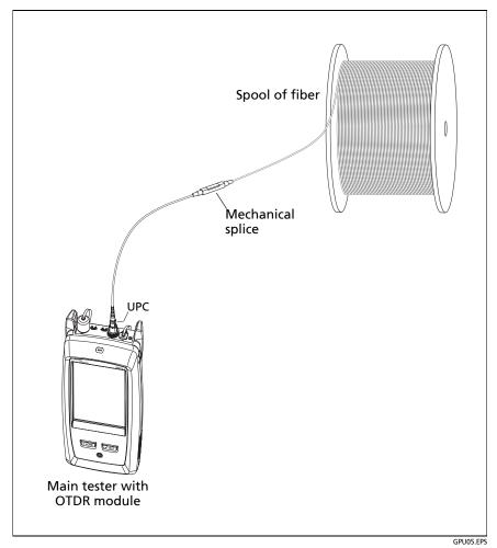
Figure 141. OTDR Connected to a Spool of Fiber
