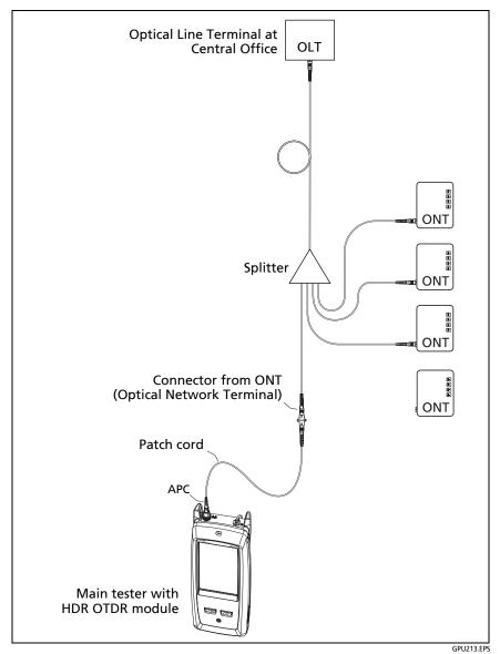
Figure 167. Typical Connections to an Out-of-Service PON Link
