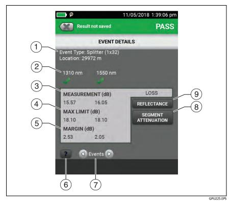
Figure 173. HDR OTDR EVENT DETAILS Screen
