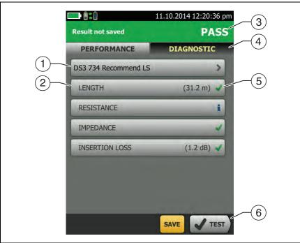
Figure 78. Autotest Results for Coaxial Cabling
