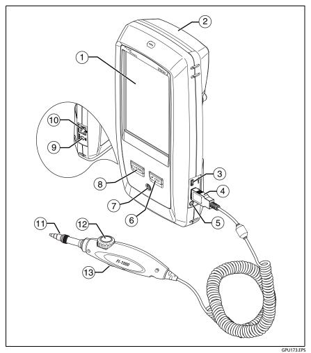
Figure 94. Connectors, Keys, and LEDs (Versiv 2 shown)
