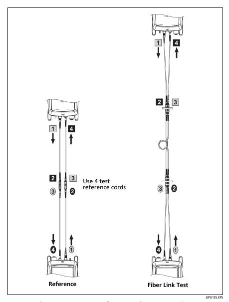
Figure C-2. 2 Jumper Reference and Test Connections (singlemode shown)
