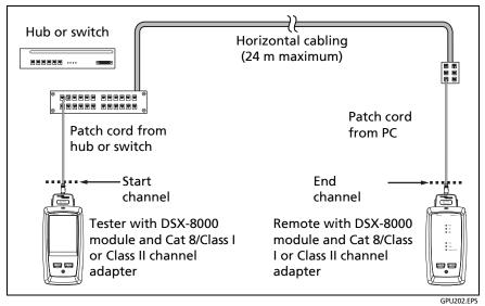
Figure 34. Channel Connections for Cat 8/Class I/II Links
