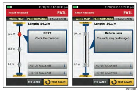
Figure 84. Examples of FAULT INFO Screens for Faults on Twisted Pair
