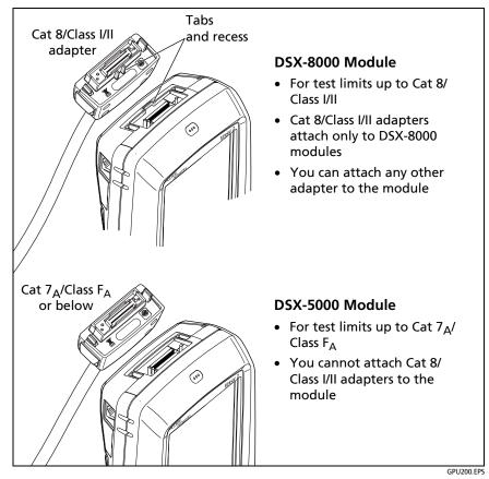
Figure 25. DSX-8000 and DSX-5000 Module and Adapter Differences
