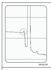
The trace shows a small reflective event with high loss. Can possibly show as an end event though it occurs before the end of the link.
