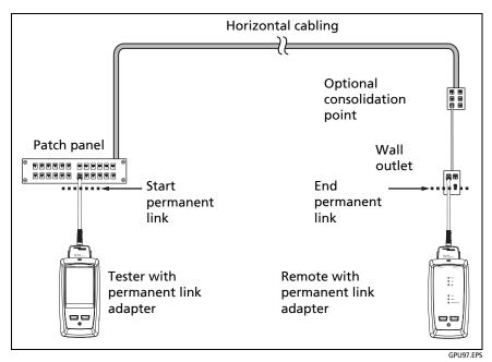
Figure 31. Permanent Link Connections for Links Up to Cat  $7_A$
