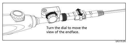
Figure 98. How to Use the Optional MPO/MTP® Inspection Tip
