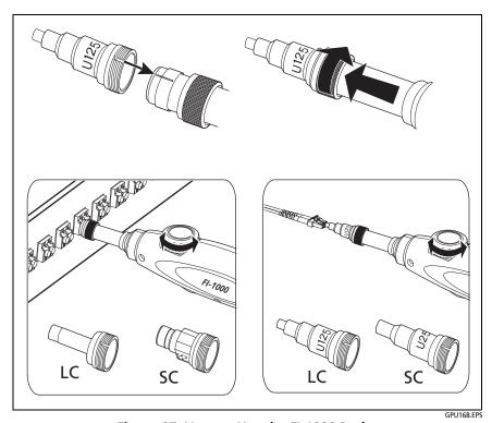
Figure 97. How to Use the FI-1000 Probe
