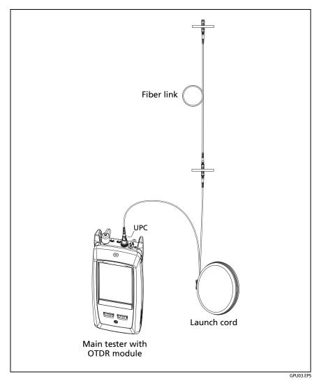
Figure 139. OTDR Connected with a Launch Cord
