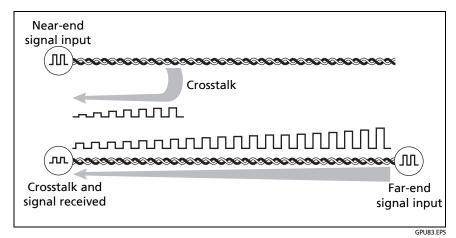
Figure 54. Attenuation to Crosstalk Ratio, Near End (ACR-N)
