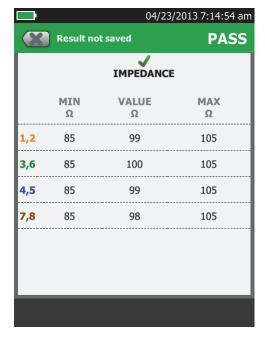
Figure 50. Twisted Pair Impedance Results
