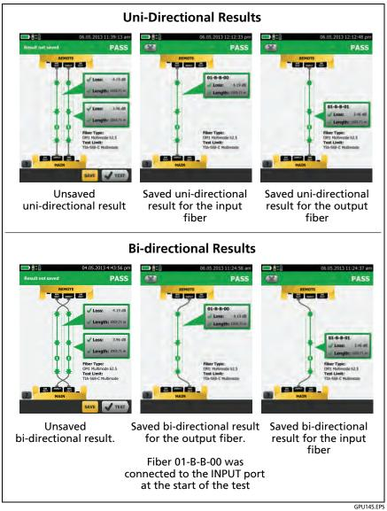
Figure 115. Unsaved and Saved Result for Smart Remote Mode
