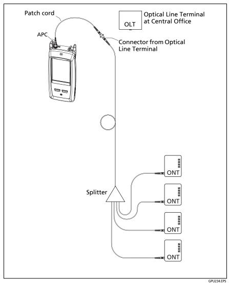
Figure 169. Typical Connections to Characterize As-Built PON Links
