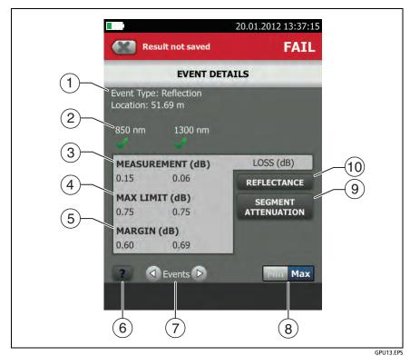
Figure 146. EVENT DETAILS Screen for a Reflection
