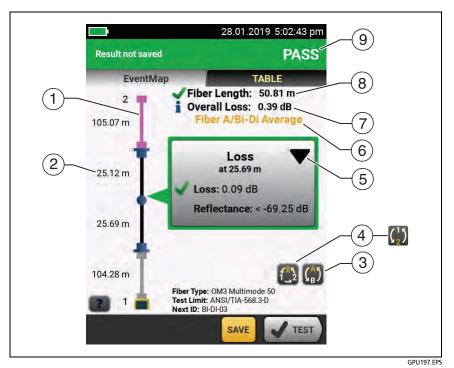
Figure 158. EventMap for Averaged, Bi-directional SmartLoop Results
