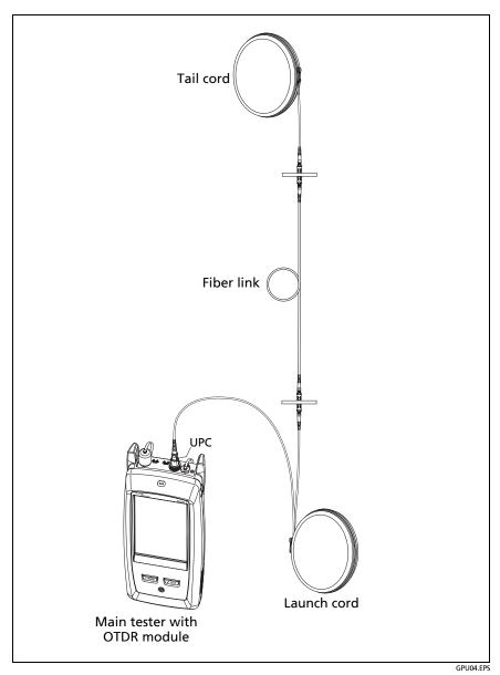
Figure 140. OTDR Connected with Launch and Tail Cords
