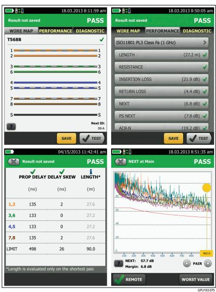
Figure 11. Examples of Twisted Pair Autotest Results Screens
