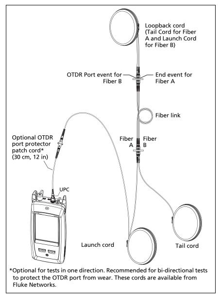
**Figure 155. SmartLoop Test Connections**
