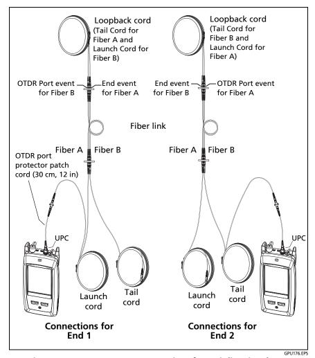
Figure 18. SmartLoop Test Connections for a Bi-directional Test
