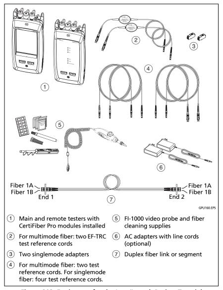
Figure 203. Equipment for the Loss/Length Project Tutorial
