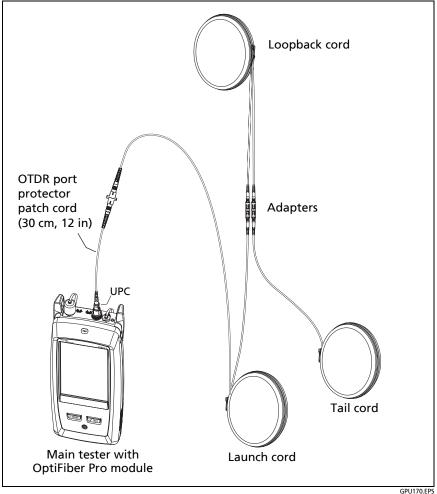
**Figure 16. SmartLoop Launch Compensation Connections**
