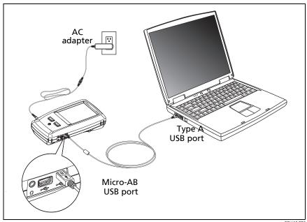
Figure 209. How to Connect the Tester to a PC
