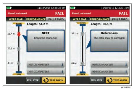
Figure 35. Examples of Fault Information Screens
