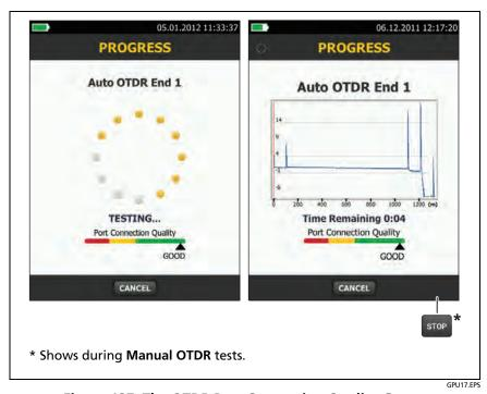
Figure 137. The OTDR Port Connection Quality Gauge and Progress Screen
