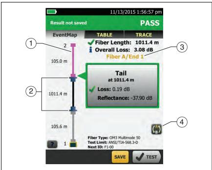
Figure 156. EventMap from a SmartLoop Test
