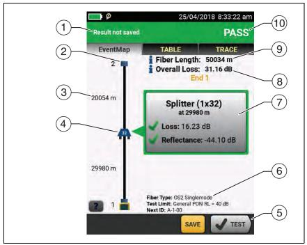
Figure 170. EventMap for an HDR OTDR Test Result
