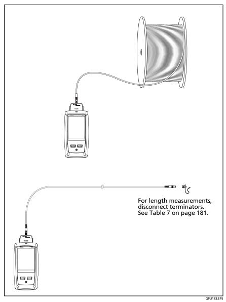
Figure 83. Connections for Coaxial Tests Without a Remote
