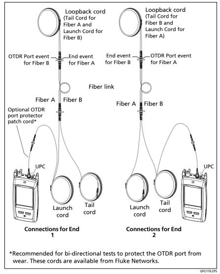
Figure 157. SmartLoop Test Connections for a Bi-Directional Test
