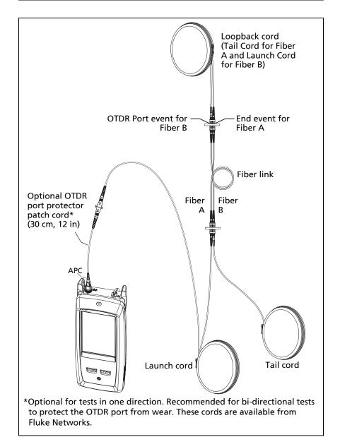
**Figure 184. SmartLoop Test Connections**
