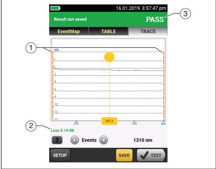
Figure 191. OTDR Trace for a Span
