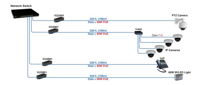
The Vi22401 can provide up to 60W PoE power to high power IP cameras or other PoE devices.
