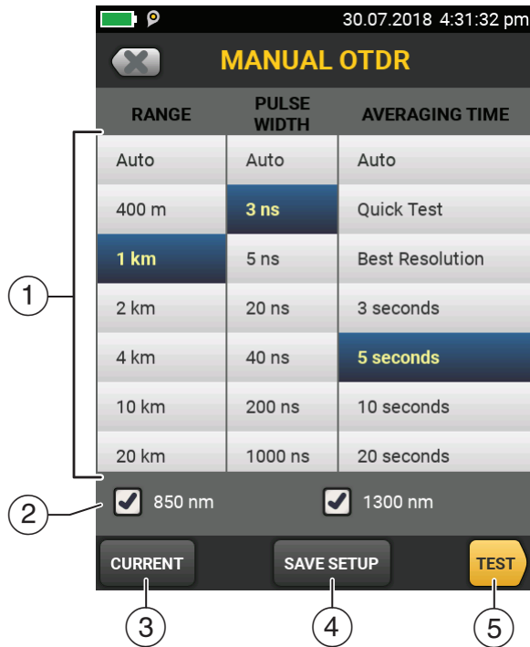
Figure 73. Manual OTDR Screen for Quick Changes After a Test
