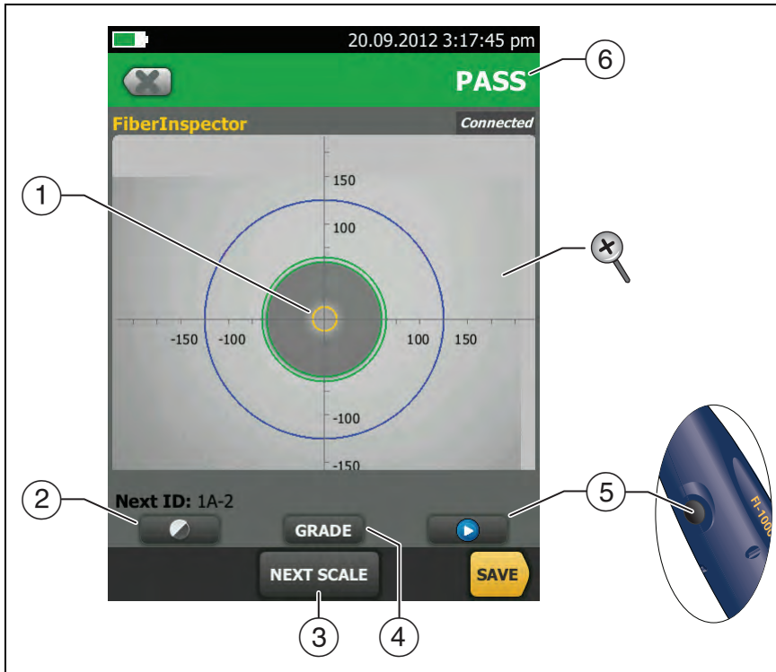
Figure 38. FiberInspector Image with Manual Grading Selected
