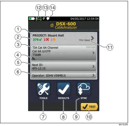
Figure 14. The Home Screen for DSX-600 CableAnalyzer
