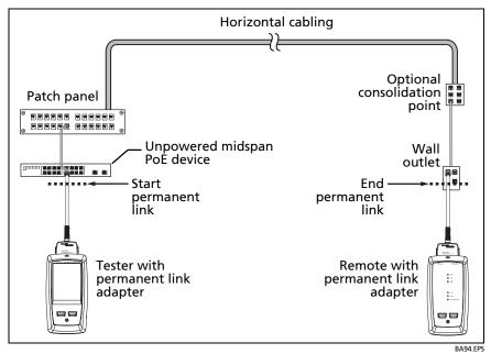
Figure 47. Permanent Link Connections Through a PoE Device
