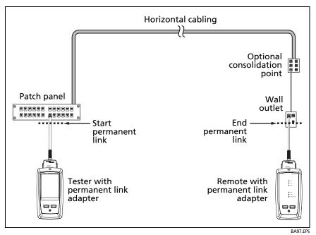
Figure 18. Permanent Link Connections
