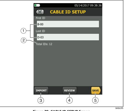
Figure 70. CABLE ID SETUP Screen (after you enter the first and last IDs)
