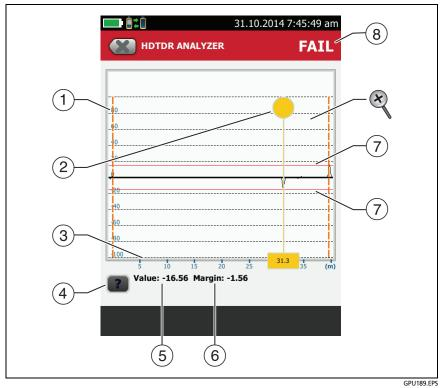
Figure 62. HDTDR Plot for Coaxial Cable
