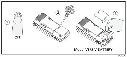
Figure 77. How to Remove the Battery
