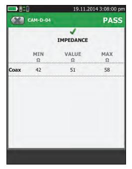
Figure 57. Coaxial Impedance Results
