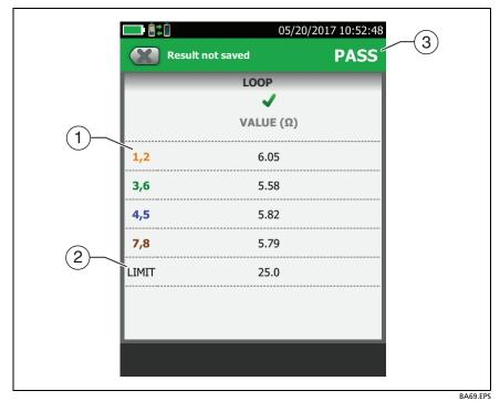
Figure 27. Twisted Pair Resistance Results
