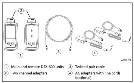
Figure 11. Equipment for the Twisted Pair Certification Tutorial
