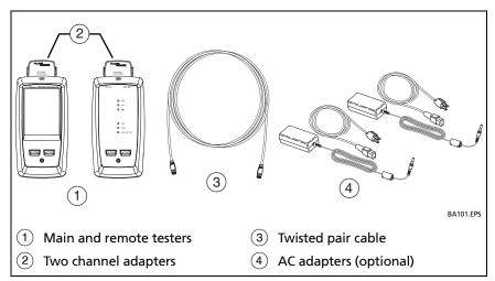
Figure 71. Equipment for the Twisted Pair Project Tutorial
