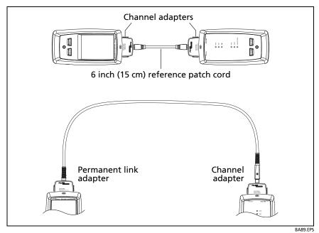
Figure 15. Reference Connections for Twisted Pair Cable
