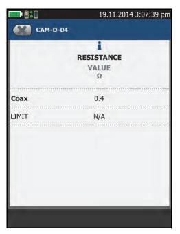
Figure 56. Coaxial Resistance Results
