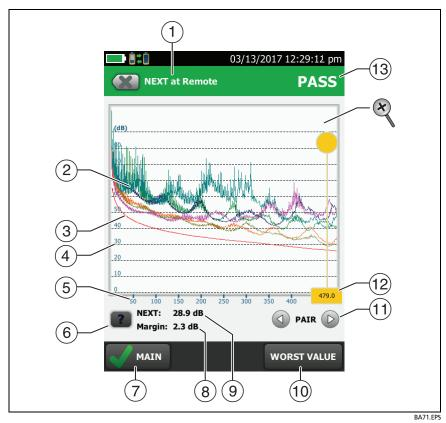
Figure 28. Plot Screen for a Frequency-Domain Test
