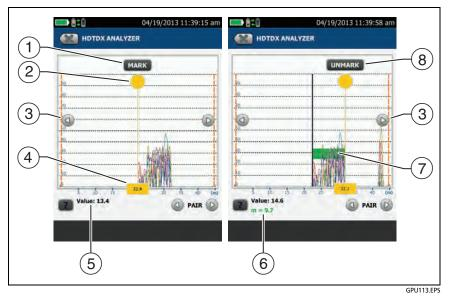
Figure 65. How to Use the Measurement Cursor on the HDTDR or HDTDX Plot
