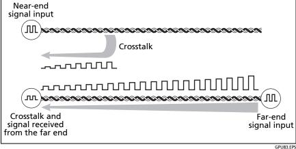
Figure 38. Attenuation to Crosstalk Ratio, Near End (ACR-N)
