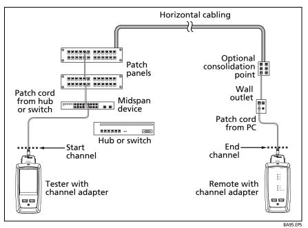
Figure 48. Channel Connections Through a PoE Device
