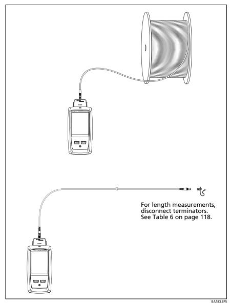
Figure 59. Connections for Coaxial Tests Without a Remote
