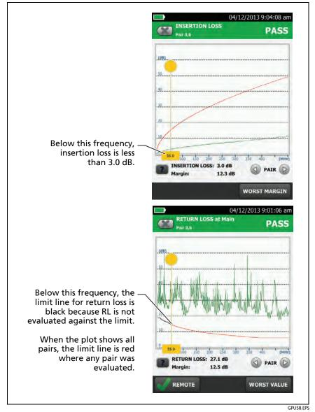
Figure 45. How the 3 dB Rule Shows on Plots
