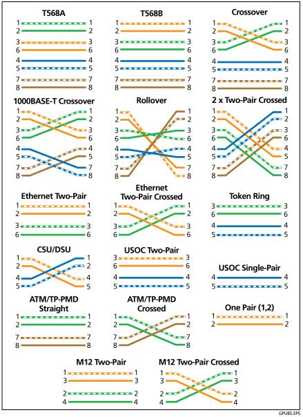
**Figure 16. Outlet Configurations**
