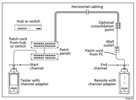
Figure 19. Channel Connections
