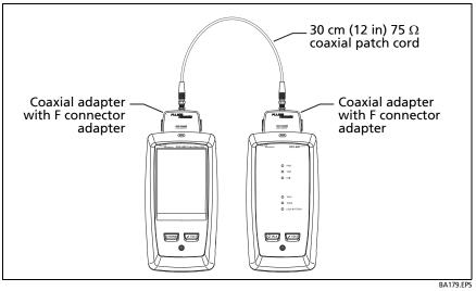
Figure 51. Reference Connections for Tests on Coaxial Cabling
