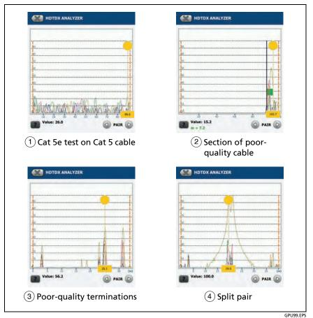
Figure 64. Typical Faults Shown on HDTDX Plots
