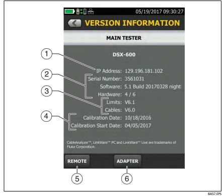
Figure 74. VERSION INFORMATION Screen for the Main Tester
