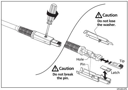
Figure 78. How to Replace the DSX-PLA004 Adapter's Tip and Latch
