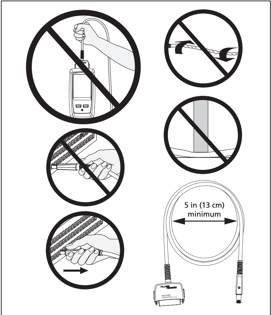
Figure 24. How to Prevent Damage to the Permanent Link Adapter Cables
