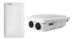
The compact and robust form factor of Tsunami<sup>®</sup> Multipoint 820 series is an ideal solution for urban wireless deployments. It is eminently suitable discrete mounting in city streets and offers high reliability for the connection of Video Surveillance, traffic monitoring and traffic light management systems.
