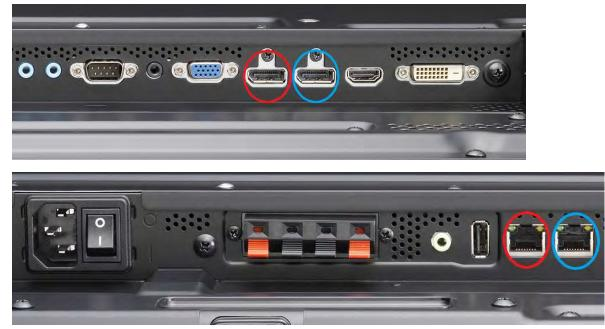
• Red circles in the above interface connections signify the IN of that particular connector. Blue circles in the above interface representations signify the OUT for that particular connector.
