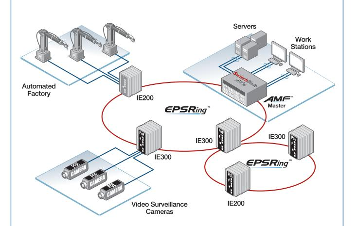
EPSRing<sup>™</sup> and ITU-T G.8032 provide high speed resilient ring connectivity. This diagram shows the IE Series in a double ring network topology.
