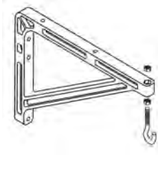
No. 11 Wall Bracket Screen can be extended 10" or 14" from wall by changing position of bracket.
