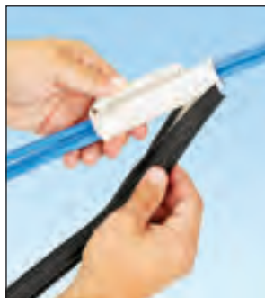
Insert Pan-Wrap™ Braided Sleeving onto end of tool until approximately 3" of it covers the bundle.
