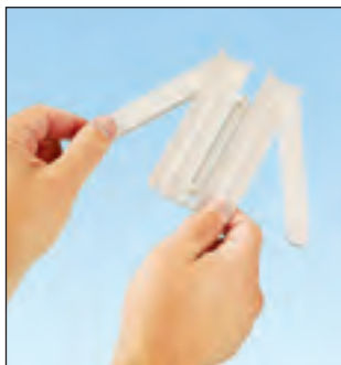
Open Pan-Wrap™ Tool and insert bundle.
