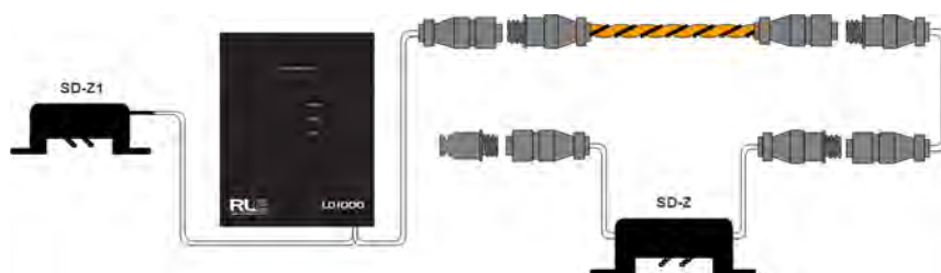
Spot detector example: use the SD-Z and SD-Z1 in conjunction with an RLE SeaHawk leak detection controller.
