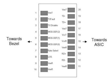
Pin-out of connector Block on Host board
