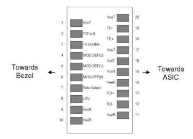
Pin-out of connector Block on Host board
