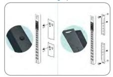
InfraPower PDUs are supplied with 2 types of mounting kits; Vertical Button Mounting Kit & Vertical Bracket Mounting Kit. The tool-less kits can be used on the majority of global branded racks.
