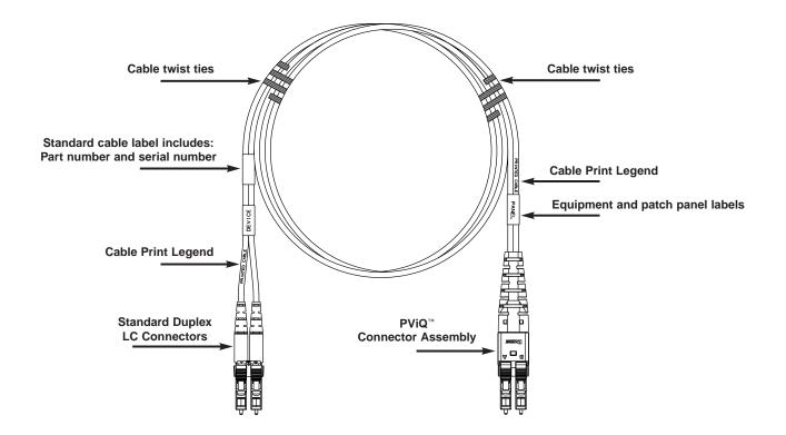
**Example Description: PVQ9PE10LQM05.0** = PanView<sup>™</sup> Interconnect Fiber Patch Cord, 9/125µm singlemode, OFNP 1.6mm jacketed, standard duplex LC – to – PanView<sup>™</sup> Duplex LC, 5.0 meters long
