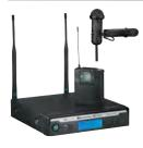
The R300-L system includes the metal BP-300 bodypack transmitter, which uses two AA batteries. With ClearScan and EZsync, the R300-L is the easiest wireless system you will ever use for presentations and worship services. The directional ULM18 helps to reject noise from the surroundings and control audio feedback.
