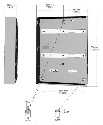
The enclosure is designed for installing two devices (AMC2 or AMC2 xl-xO-EXT), two power supplies (AMC PBC60) and two batteries.
