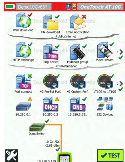
Figure 10: Group tests by target location - local, intranet, internet. (OneTouch AT 10G Test result shown).
