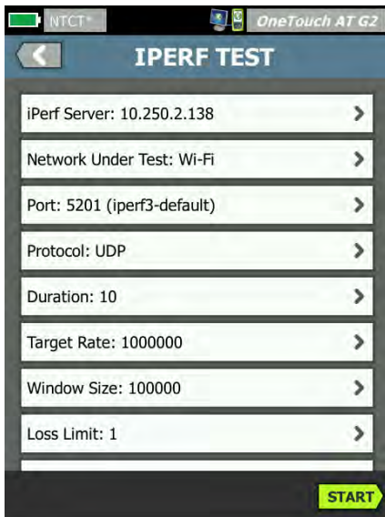
Figure 21: Setup for TCP Window Size and Threshold.
