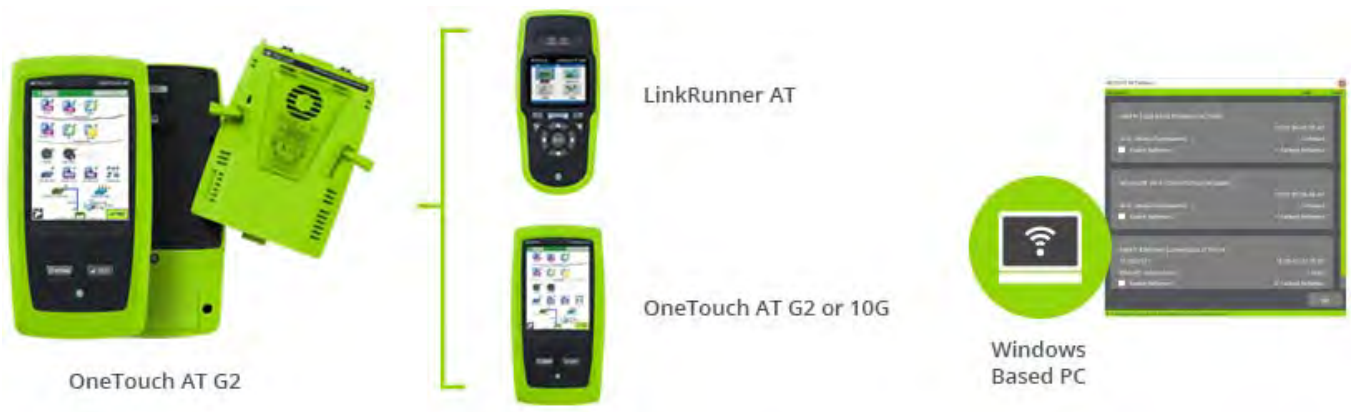
Figure 15: NPT Tests through its Wired or Wi-Fi test port against several types of remote end-points.
