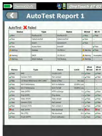
Figure 32: Detailed breakdown of the PDF report on network service performance which can be viewed on the unit itself or uploaded to Link-Live.
