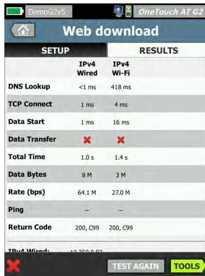
Figure 9: Detailed breakdown of network-hosted application performance including return code of web transaction. This level of detail allows quick isolation of issues when tests fail.
