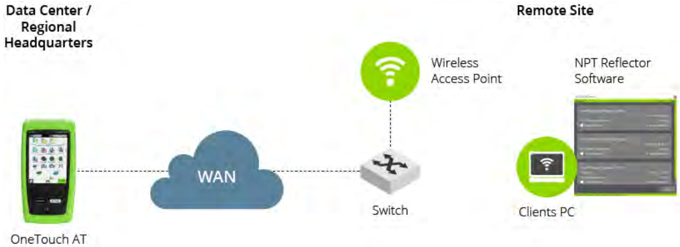
Figure 14: The NPT Reflector can be downloaded directly from OneTouch G2 or 10G to a Windows PC at a remote site to validate network performance.
