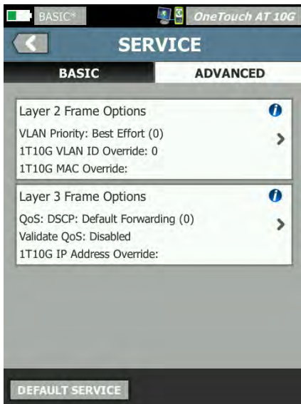
Figure 18: 10G NPT tests allows users to override VLAN, MAC, IP address and the class of service.
