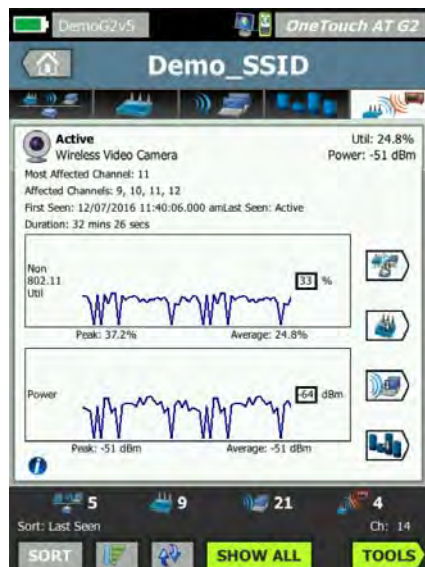
Figure 26: Detailed information about a specific interference source.
