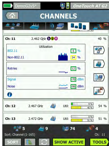
Figure 24: Visibility into each Wi-Fi channel, showing bandwidth occupied by 802.11 and non-802.11 traffic.
