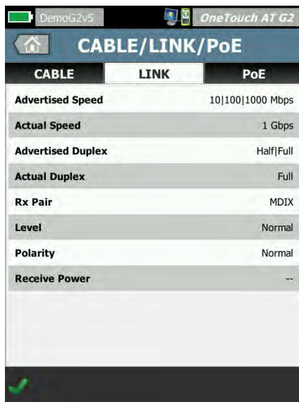
Figure 4: Test link speed over twisted pair and fiber-optic links at rates up to 1 Gbps and measure PoE voltage with the G2 Module.
