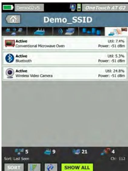
Figure 25: Unique Interferer analysis classifies sources of non-802.11.
