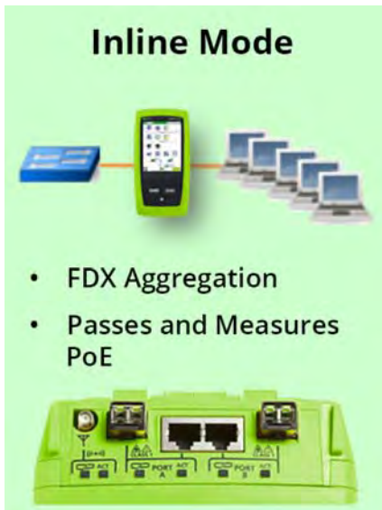
Figure 29: Inline packet capture simplifies documentation of client application problems without TAPs or SPAN ports.
