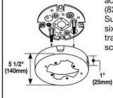
Fan Box/Solid Base – UL approved fixture box for ceiling fans. Cover accepts fan brackets with 3.2" (82mm) mounting centers. Supports up to 50 lbs. Base has six mounting holes and four 1/2" trade size KOs. #10 mounting screws provided.
