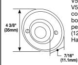
Blank Cover – Use with V5735, V5737, V5737A, V5738A, V5738, or V5739A, or V2135 converting them to pull or junction boxes and for hanging lightweight pendant fixtures having 1/2" (12.7mm) pipe stems, etc. Has 1/2" trade size KO.
