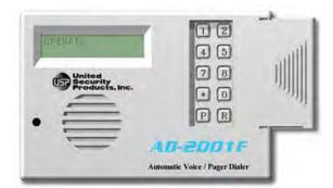
The AD-2001F dialer features busy-line and no-answer detection to ensure prompt transmission of up to 2 prerecorded messages delivered sequentially to as many as 4 standard telephones, cellular phones, voice and/or numeric pagers. Messages to both local and long-distance calls can be transmitted. When activated, the dialer instantly begins calling the numbers in sequence, delivering each message 1 to 3 times in a row, in accordance with the preselected number of dialing attempts.
