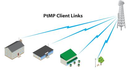
NanoStationM used as powerful clients in an airMAX PtMP (Point-to-Multi-Point) network setup.
