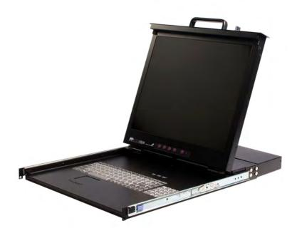
The RACKCONS1908 1U 19-inch Rack Mount LCD Console provides centralized control for servers and KVM switches with an integrated 8-port KVM switch, a 19-inch LCD monitor, full 106-key keyboard and touchpad, neatly combined into 1U of rack space for any standard rack or cabinet 30-inches (or greater) in depth.
