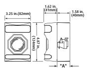
Covers to protect your STI Stopper Station from damage or weather and to help stop malicious or accidental activation.
