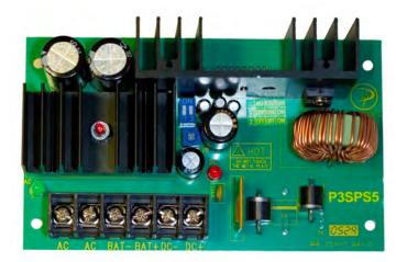
The P3PS-5 is a switching power supply and charger. It is engineered to convert low voltage AC input into 12 VDC or 24 VDC @ 5 AMPS of continuous supply current.
